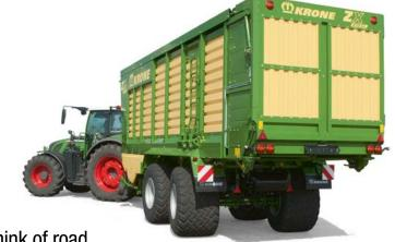
and field safety. Therefore, KRONE offers an electronic brake system that has already proven its worth on our commercial trailers. Steered axles help protect the swath and provide added safety.
