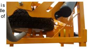
This drive system has the advantage of the operator being able to apply a variable tension to the wire from very high force to pull wires through long rows of tomato trellis with entangled growth, through light strain when the end of the wire is near.
