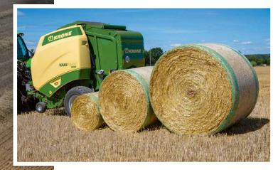
KRONE VariPack is a belt baler that was specifically designed for baling dry crops. The design focuses on simple technology, high throughputs and high baling densities.
